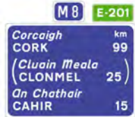
Route confirmatory sign with Euro Route marker plate
