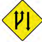
Start of a climbing lane
