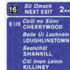
Typical 2km next exit sign
