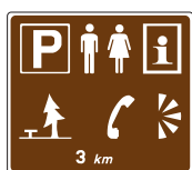
Advance sign for facilities in lay-by
