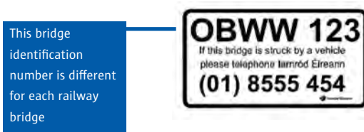
Example Railway Bridge Identification Plate
