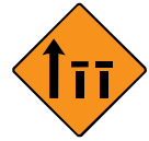
Two offside lanes (of three) closed
