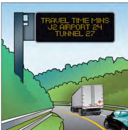
Typical LED VMS
